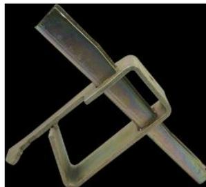
**WASHER TIE:** A snaptie with a metal washer used to stabilize a tie in a form in the place of a cone tie.
